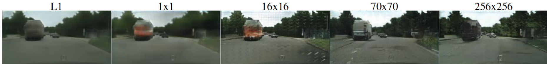
Figure 6: Patch size variations. Uncertainty in the output manifests itself differently for different loss functions. Uncertain regions become blurry and desaturated under L1. The 1x1 PixelGAN encourages greater color diversity but has no effect on spatial statistics. The 16x16 PatchGAN creates locally sharp results, but also leads to tiling artifacts beyond the scale it can observe. The 70x70 PatchGAN forces outputs that are sharp, even if incorrect, in both the spatial and spectral (cofornfulness) dimensions. The full 256x256 ImageGAN produces results that are visually similar to the 70x70 PatchGAN, but somewhat lower quality according to our FCN-score metric (Table 2). Please see https://phillipi.github.io/pix2pix/ for additional examples.
